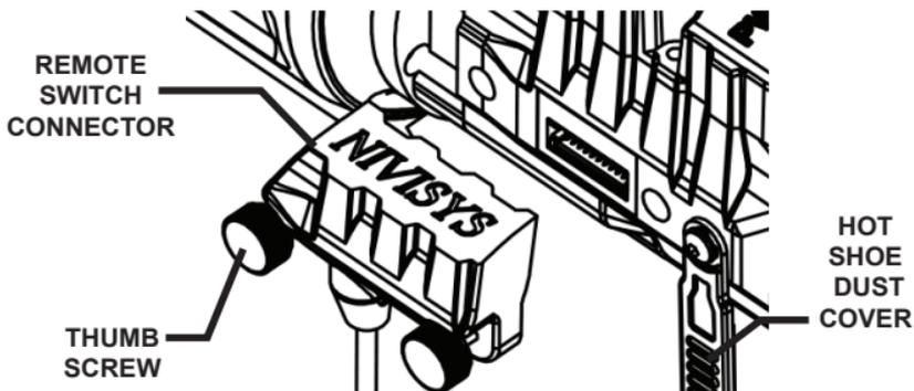
Figure 2-17 Remote Switch Installation
