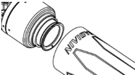
Figure 2-2 Hood Installation Alignment
