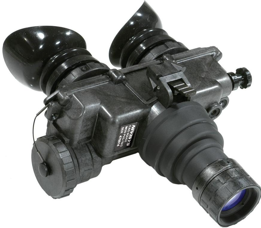
The PVS-7B/D is the standard issue goggle for U.S. ground forces to conduct night operations. Using the latest GEN II or GEN III image intensifier tubes the PVS-7B/D will perform in the darkest of nights. The system has a built-in IR Illuminator for no light operations and a highlight cut-off sensor to protect the image intensifier in case of extended exposure to high light conditions. The PVS-7B/D is a completely MIL-SPEC system that has been ruggedized and waterproofed for harsh environments.
