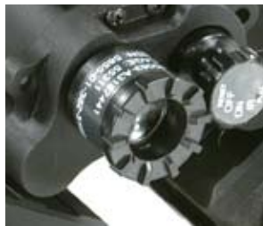
Built-In Illuminator IR-LED illuminator
