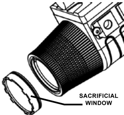
Figure 2-5 Sacrificial Window Installation
