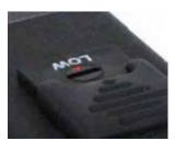
**Eye-Safe Selector** The GCP-1 is equipped with a selector switch that allows for an eye-safe training mode.
