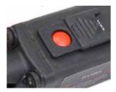
**Momentary Switch** A robust switch is featured on the unit for use with or without gloves.
