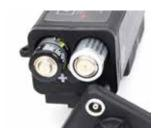
**Battery Power** The unit's power operates on two AA alkaline or lithium batteries.
